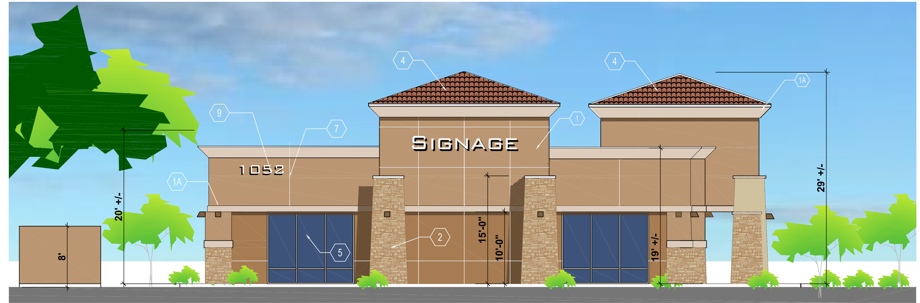
2 South Elevation Scale : 1/8" = 1'-0"
